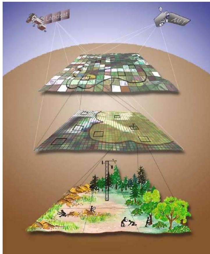
Figure 3.9. Conceptual model from the Bigfoot project. illustrating the use of field measurements and remote sensing to characterize the vegetation cover and LAI for study sites ( http://www.fsl.orst.edu/larse/bigfoot/ ).
