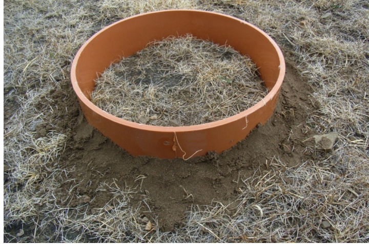
Figure 5-1: Soil collar for soil CO 2 flux measurements, sealed with silt against boundary effects
