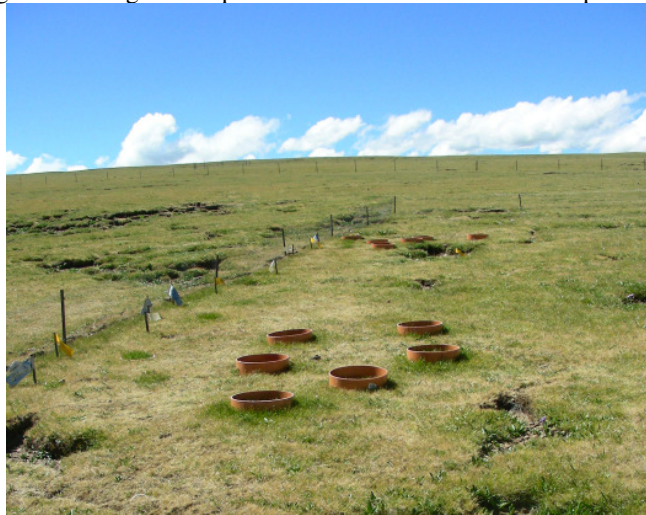
Figure 9-1: Block design of the irrigation experiment on a herbivore exclusion plot
