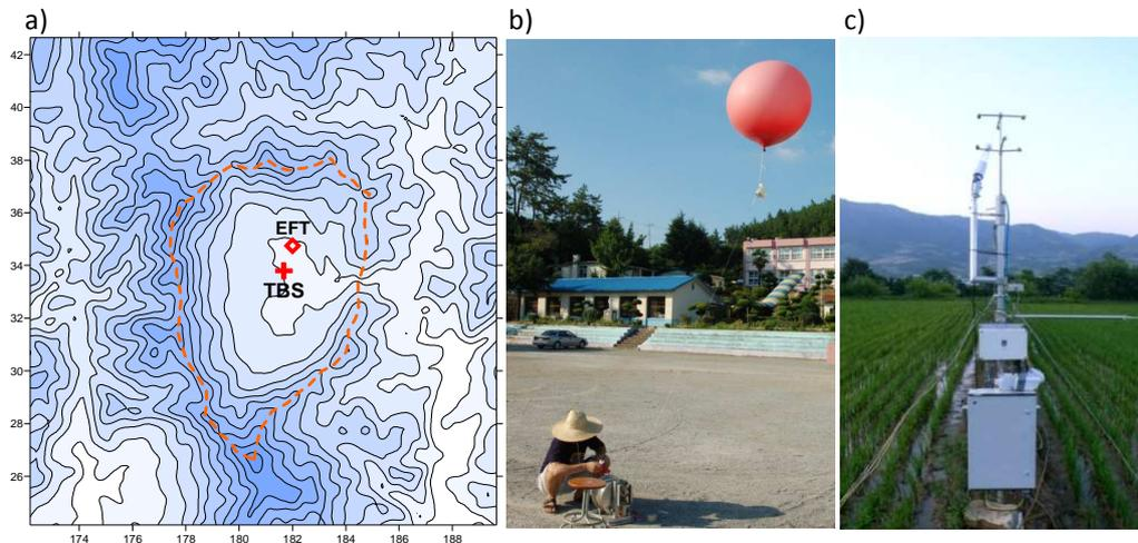
Figure 1. a) Location of tethered balloon sonde experiment (TBS) and eddy flux tower (EFT). b) tethered balloon sonde (photo by Miloslav Belorid) c) eddy flux tower (photo by Zhao Peng)
