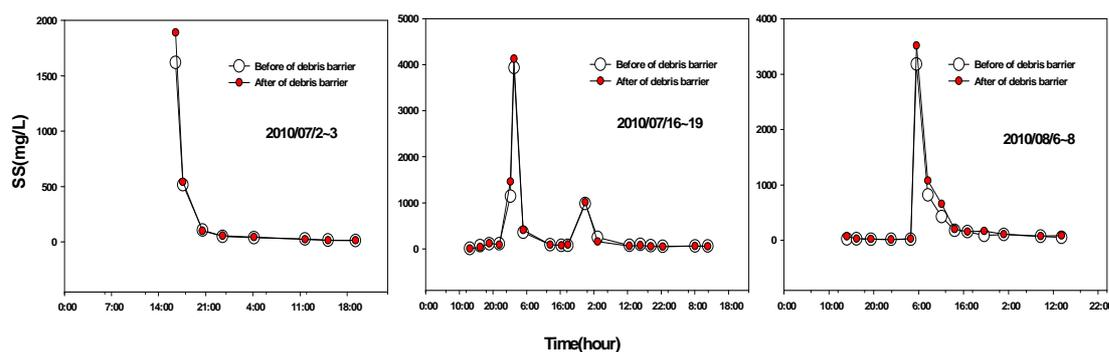
Figure 2. The removal efficiency of TSS by debris barrier during storm events
