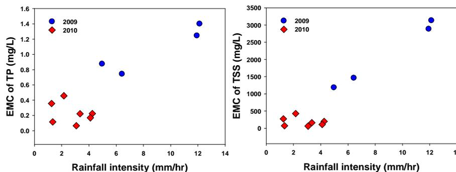
Figure 4. Comparison of EMC of TP and SS in the Naedong stream according to rainfall intensity
