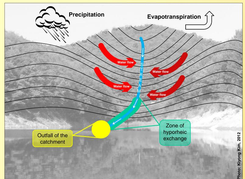
Figure 2. Graphic representation of a simplistic conceptual model of water flow within a forested catchment.
